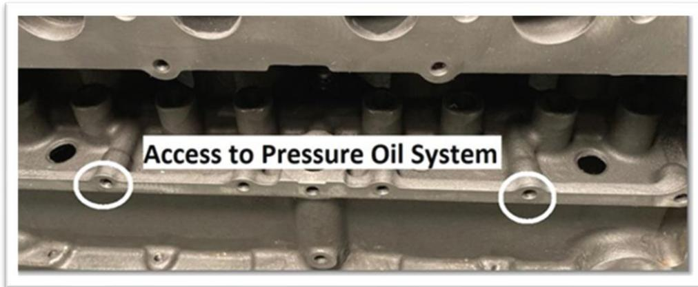
Oil Galley Plugs: There are 5 oil galley plugs that must be in place to maintain oil pressure.
